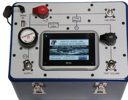
This unit has two flow ranges and two pressure channels. The 1402 quantifies the component's leakage rate by maintaining a constant gas pressure against the barrier being tested while measuring the gas flow rate needed in order to maintain that pressure constant.
