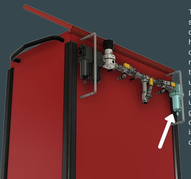
The Inline moisture trap, water separator filter. Removes water droplets and moisture which will help prevent potential contaminated water from returning in to the LRM. Designed to be used in compressed air lines up to 150 PSI variable test pressure, air flow is completely unrestricted. filtration works on a gravity fed principal. Easy to use drain attached to the bowl which is protected by an impact resistant casing.
