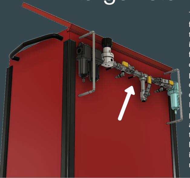
This manifold allows for the quick filling of large volumes. The tainless steel manifold incorporates a 1/2" pipe, welded fittings and ¼ turn ball valves. This device allows for quick pressurization, testing as well as quick depressurization while completely bypassing the Leak Rate Monitor. This not only prevents equipment damage it also drastically cuts down test times. saving in average about one hour from each test. Less man time in the RCA equals less dose and results in ALARA savings.
