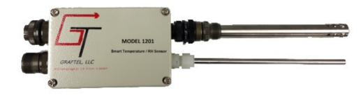
The RS-485 network allows for multiple sensors to be connected to a PC's communications port with a single 4-wire cable string. A typical ILRT may use six strings with seven or more sensors per string. Although the are physically connected in series, they are electrically connected in parallel so that the failure of any one will not affect the others.
